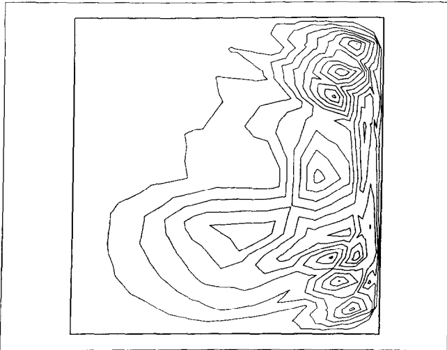
FIG. 28. Contours of E calculated on the grid shown in Fig. 27, E_{max} is at (x, y) = (0.87, 0.83) .
